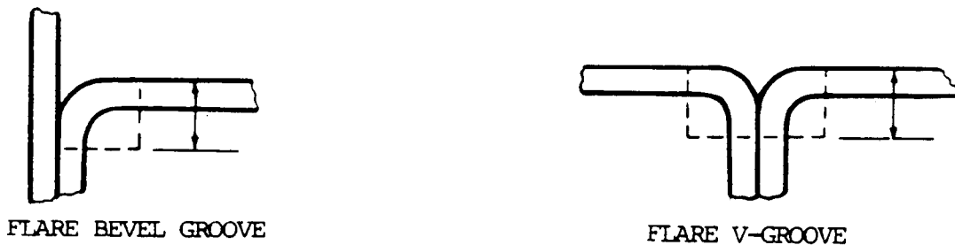
Figure 3-48. Flare groove welds.
