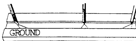
Figure 6-61. Effect of ground location magnetic arc blow.
