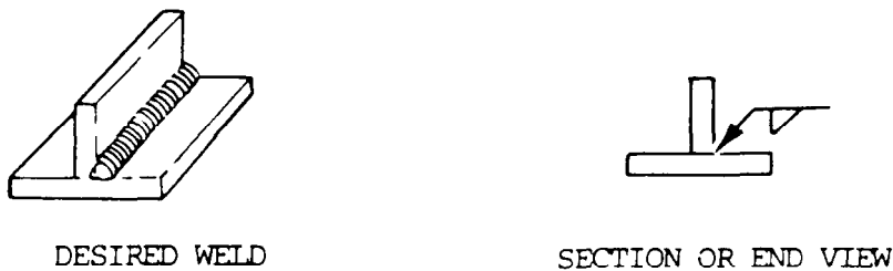
Figure 3-9. Arrow side fillet welding symbol.
